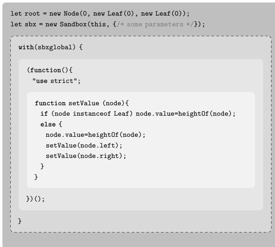
■ Figure 10.3 Scope chain installed by the sandbox when loading setValue . The dark box represents the global scope. The dashed line indicates the sandbox boundary and the inner box shows the program code nested inside.
